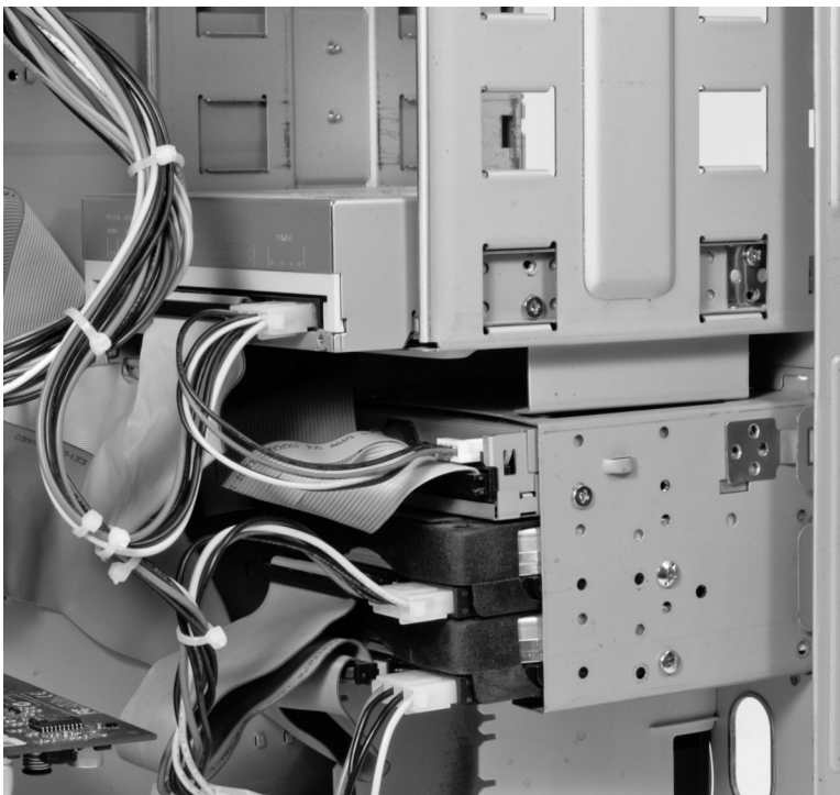
FIGURE 3-12 Typical drive configuration in a PC tower system case; note the cages or frames used for mounting the various drives
